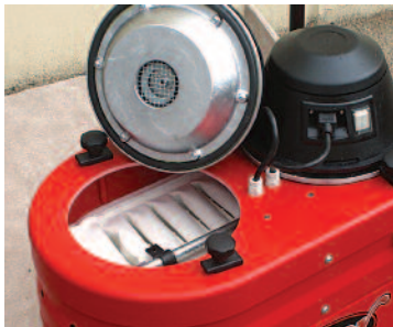
Motors are easily removed for service
